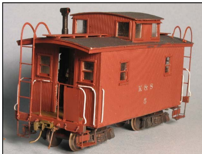
Fig. 1: The painted caboose before final weathering. The end ladders are held down by brass pins in the end beam and roof. A functioning door is simply hung on paper hinges, held with styrene cement.
