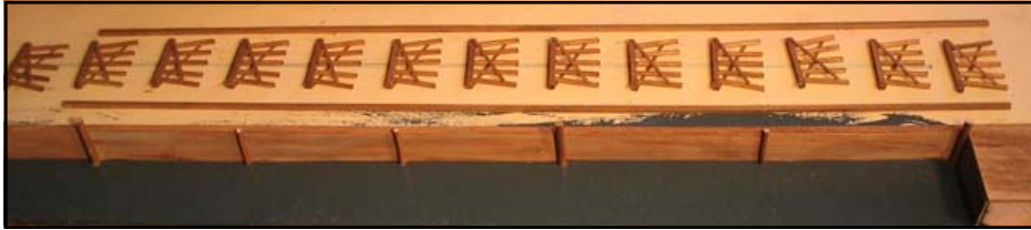
Fig. 5 Above: Half the required bents are in this view as are the two stringers for this section of the trestle.
