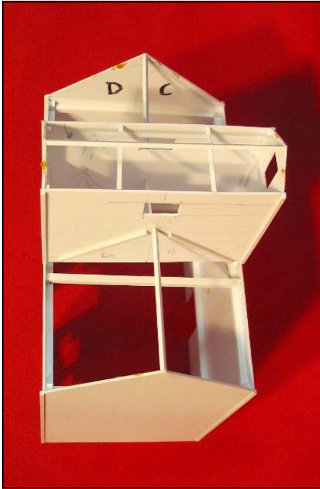
Figure 6: Canopy. The completed canopy sub-assembly illustrating the various 6x6 strip styrene bracing as described in the text. Note as well the triangular clapboard piece on the ends.
